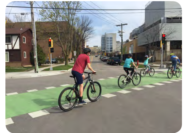
ABOVE: Crossing treatment at signalized intersection along bike trail. A similar treatment could be used to direct bicycles across Tayco Street to Main Street. BELOW: The crossing treatment on Main Street is one example of how the City might address the proposed pedestrian crossing at the Tayco Street bridge.
